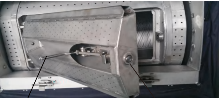
left right moveable single door large door opening, convenient for loading & unloading, no barrier panel, much cleaner after washing
